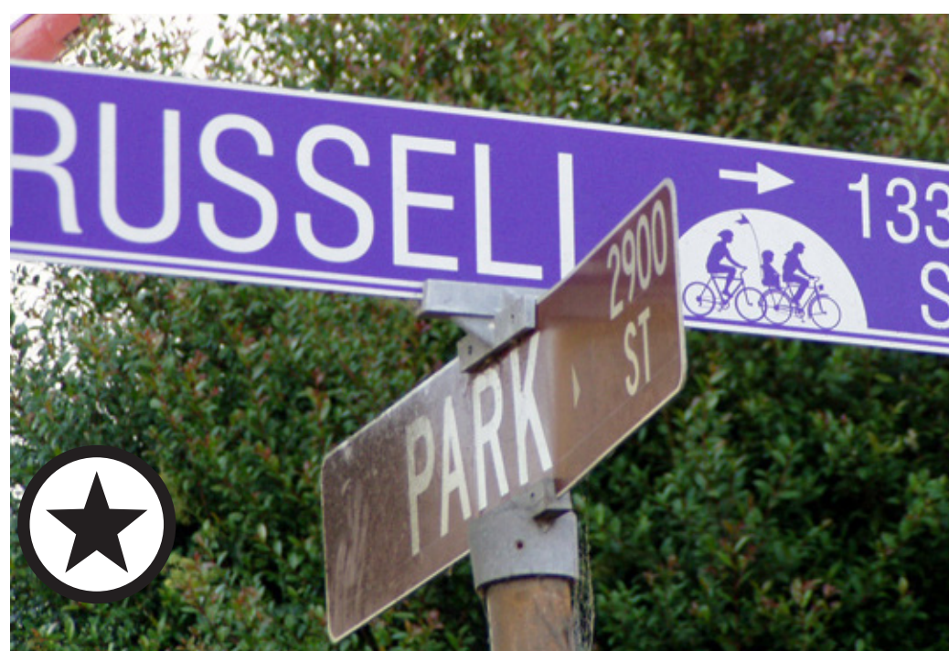
Street signs can be used to indicate that the street is a bicycle boulevard. Credit: NACTO
