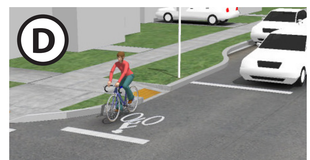
A bicycle forward stop bar, used in conjunction with a curb extension, improves bicyclists' view of cross traffic. Credit: NACTO
